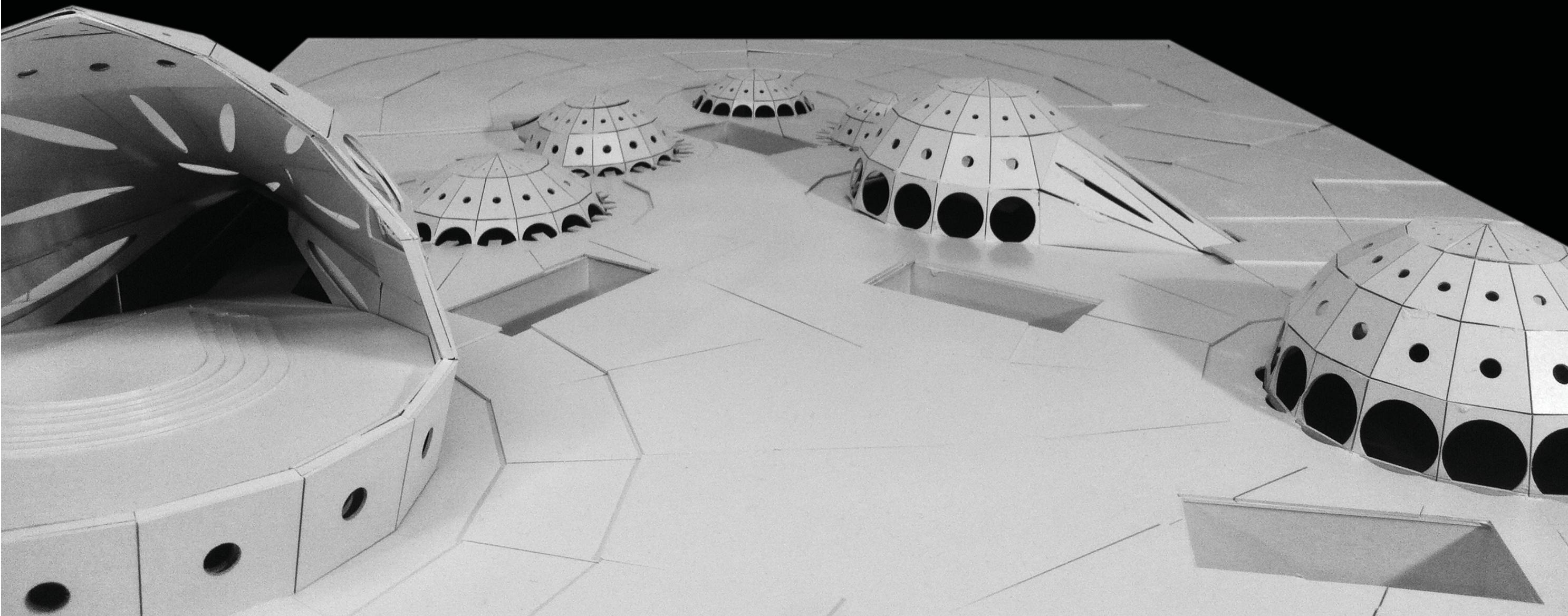
*MODEL FLOOR PLATE SECTION:* This section of the model further illustrates the area between the theaters on each floor plate where the office, support, and other non-theater program exist. The idea of theatricality is extended beyond the theater onto the office floor space by creating stepped areas for program. The balconies of the workspace extend into the theater creating a new type of office zone that becomes theatrical as workers become the spectators of the theater.
